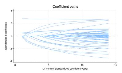
We see four lines that do not start at 0. These are lines corresponding to the four variables in idemographics that we forced into the model.
